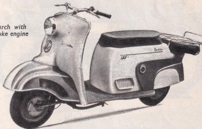
Two-stroke twin: the 244 c.c. Excelsior Talisman
